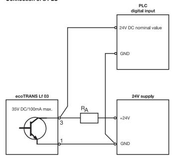
$R_A$  is a current-limiting resistor for I = 100 mA max.
