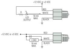
Note: Inductive loads must be diode suppressed.
